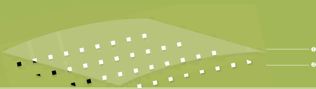
1 transparent PVC film 2 printed backing & standard coating
